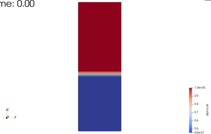
twoPhaseEulerFoam Air volume fraction Laminar case
