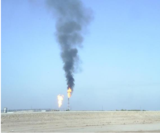
Large Natural Convection Plume, as effect of combustion of excess non-useable gases behind oilfield.
