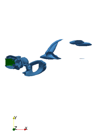
RANS (K-Omega SST) – Vortices visualized by Q-criterion
