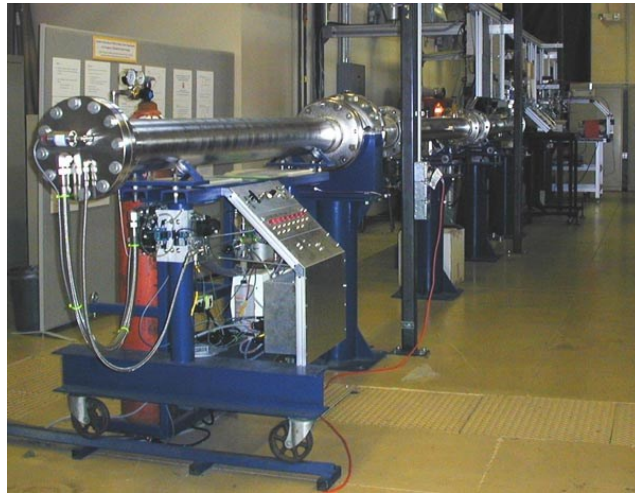
Shock tube. The driver section, including vacuum pumps, controls, and helium driver gas. Photo credit: Stanford University. http://hanson.stanford.edu/index.php?loc=facilities_nasa Copyright on the images is held by the contributors. Apart from Fair Use, permission must be sought for any other purpose.
