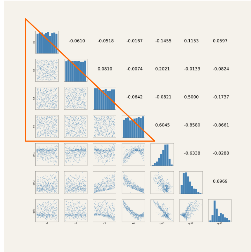
Scatter matrix plot of the design space exploration study – 600 experiments (high fidelity simulations) Scatter plot of design variables distribution (sampling distribution in design space)
